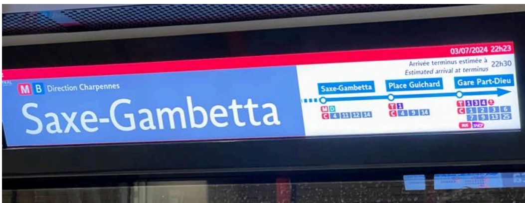
Image of an LCD Screen Installed on a Metro B Vehicle
